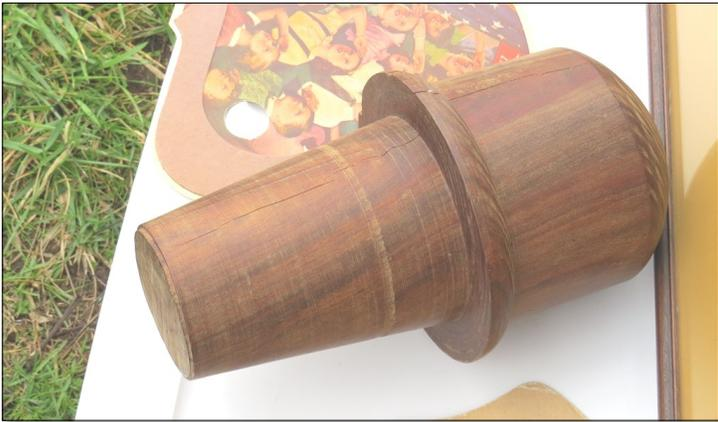
It is the bottom bearing for a turbine, made of a very hard wood, Lignum Vitae, from the Caribbean. The wood has natural oils that self-lubricate as it wears away. The turbine runner has a cup on the bottom that rests on the rounded top of the bearing. Below is a picture of a bearing as it would be positioned in the bottom frame of a turbine.
