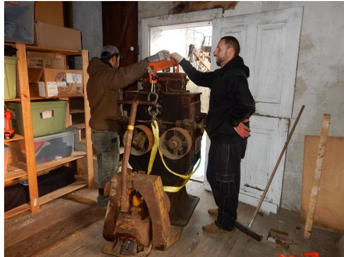
Photo 1: Careful rigging was required to assure that the full weight of the roll stands was carried on the cast base with no force applied to the bearings or wooden feeder section
