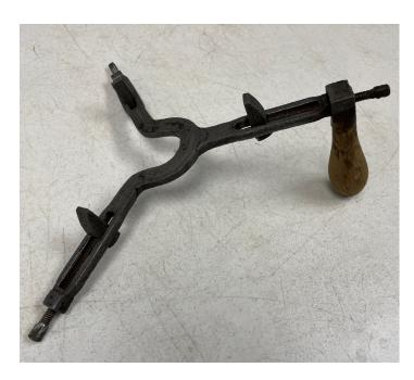
Mystery Tool: The bit on each of the three legs is adjusted to securely clamp the end of a wooden water wheel shaft so the handle can be used for manual rotation while making repairs.
